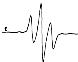
Fig. 1c. Cw ESR first derivative spectrum observed during the photolysis of DTBQ and hexamethyldisilane at 23 °C;
